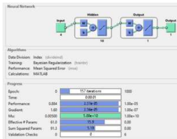
Fig. 10. Neural Network Training Progress and Configuration in MATLAB.
