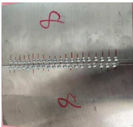
(b) Work piece for FSW process with micro drilling
